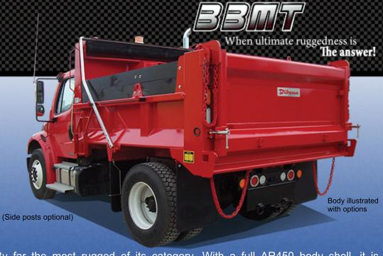
By far the most rugged of its category. With a full AR450 body shell, it is unquestionably the best suited to sustain constant abuse (heavy duty excavating, demolition). Furthermore, the AR steel provides this body with an incomparable wear-resistant factor as well as the ultimate resistance to impacts.
