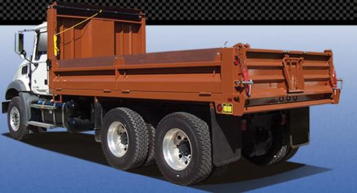
If your application requires easy side and rear access, the MS0-2 & the MS0E-2 are for you. The two drop sides combined with the double-acting door, greatly increase their versatility. The grade 50 steel used in their respective construction, provides both models necessary ruggedness to do the job while maintaining weight to a minimum.
