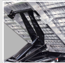
Champion Hoist Installed
