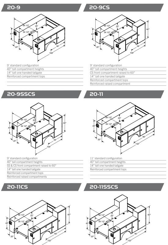
11' standard configuration 40" tall compartment heights CS front compartment raised to 60" 14" tall one handed tailgate Reinforced compartment tops Reinforced raised compartment
