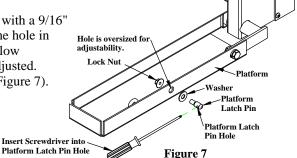
Center the platform latch pin vertically in the latch hole. Push the platform latch pin toward the front of the truck so there is a 1/8" gap (Page 10, Figures 10& 11) . Tighten the platform latch pin with a 9/16" wrench and a screwdriver.
