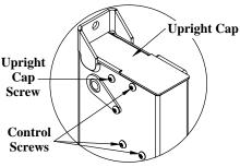
**Figure 5.** Remove the upright cap and control screws.
