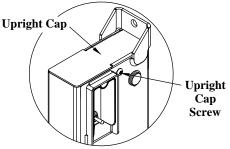
**Figure 6.** Remove the upright cap screw.
