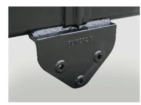
This hoist is easily installed on the trucks chassis' using extra heavy duty 4140 grade cast mounting brackets, with eight 1/2" and two 5/8" grade 8 bolts. This Subframe is built with A572 grade 50 high tensile steel & 4140 grade weldable castings
