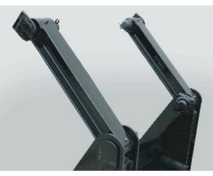
Shown is the heavy duty cast lift arms. These arms easily attach directly to the body using 4140 grade, 1 1/2" hinge pins. The arms have easily accessible zerk grease fittings.
