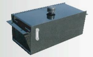
The 8.5 gallon box type reservoir is designed to be frame mounted. It hangs out of the way and is equipped with a brass wire mesh suction strainer, oil level & temperature gauge.
