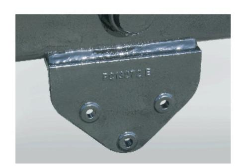
This hoist is easily installed to the trucks chassis using extra heavy duty 4140 grade cast mounting brackets. With 20 grade 8 bolts and minimal welding, installation is quick and easy.
