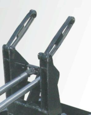
Champion built cylinders and hoists are designed to be double acting (power up and down). Our hoists are easy to install with as little truck and body modification as possible. To further ease the installation process, Champion hoists mount to the body and truck chassis using heavy duty grade 8 bolts with little or no welding needed.
