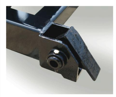
The hinges are cast 4140 grade steel to ensure durability. Adding to the ease of installation and durability, these hinges are welded directly to the body's longitudinals. cable control.
