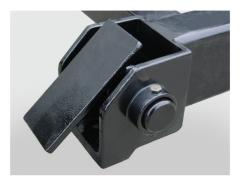
The hinges are cast from extra heavy duty 4140 grade steel to ensure durability. Adding to the ease of installation and durability, these hinges are welded directly to the body's main runners.
