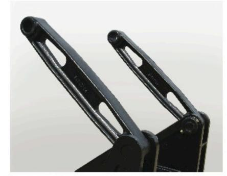
Shown is the 834SF heavy duty cast lift arms. These arms easily attach directly to the body using 4140 grade, 1 1/2" pivot pins which are bolted in place with grade 8 bolts.
