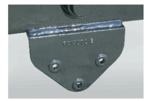
This hoist is easily installed to the trucks chassis using extra heavy duty 4140 grade cast mounting brackets. With 18 grade 8 bolts and minimal welding, installation is quick and easy.
