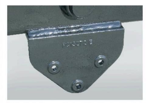
This hoist is easily installed to the trucks chassis using extra heavy duty 4140 grade cast mounting brackets. With 18 grade 8 bolts and minimal welding, installation is quick and easy. This Subframe is built with A572 grade 50 high tensile steel & 4140 grade weldable castings
