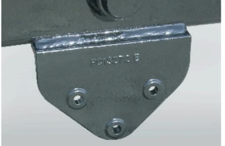
This hoist is easily installed to the trucks chassis using extra heavy duty 4140 grade cast mounting brackets. With 14
