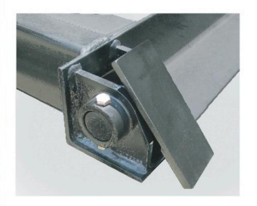
The 826Sf's hinges are cast from extra heave duty 4140 grade steel to ensure durability. Adding to the ease of installation and durability, these hinges are bolted then welded to the bodies longitudinals
