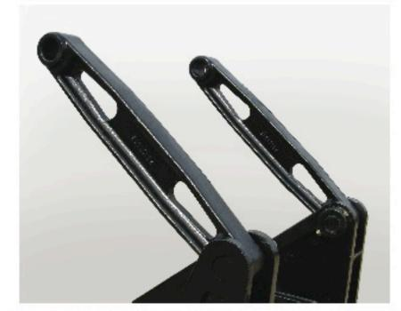
Shown is the 826SF heavy duty cast lift arms. These arms easily attach directly to the body using 4140 grade, 1 1/2" pivot pins which are bolted in place with grade 8 bolts. This Subframe is built with A572 grade 50 high tensile steel & 4140 grade weldable castings
