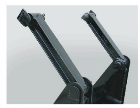
Shown is the 820SF heavy duty cast lift arms. These arms easily attach directly to the body using 4140 grade, 1 1/2" hinge pivot. The arms have easily accessible zerk grease fittings.
