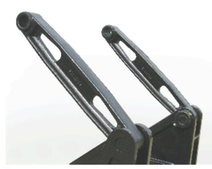
Shown is the heavy duty cast lift arms. These arms easily attach directly to the body using 4140 grade, 1 1/2" pivot pins which are bolted in place with grade 8 bolts. This Subframe is built with A572 grade 50 high tensile steel & 4140 grade weldable castings
