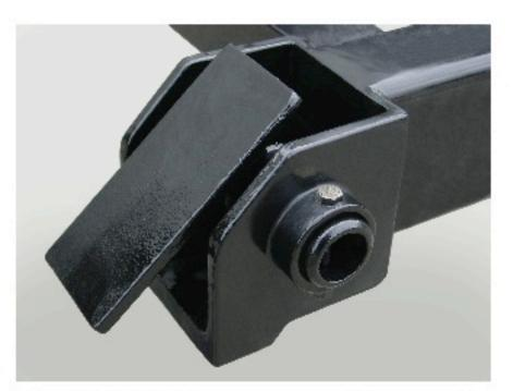
The 820SF's hinges are cast from extra heavy duty 4140 grade steel to ensure durability. Adding to the ease of installation and durability, these hinges are welded directly to the body's longitudinals.
