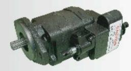
The G102D pump/valve combination direct mount gear pump does not require a drive line thus making it safer and more dependable. This pump has an S.A.E. "B" 2-bolt flange. 15 GPM @1200 RPM Available with "ccw" or "cc" rotation
