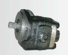
The P21 direct mount gear pump is bi-rotational with side and rear ports for versatility, thus eliminating the drive line for added safety and dependability. This pump has an S.A.E. "B" 2-bolt flange and is used for lighter duty hoists. 10 GPM @ 1200 RPM
