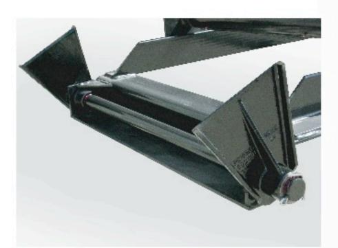
Shown are the 4140 heavy duty steel rear hinges with full length hinge pin. These hinges weld directly to the longitudinals.
