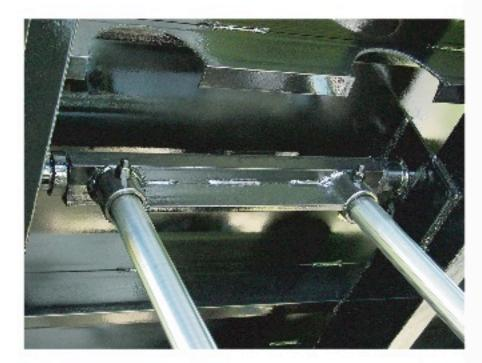
The upper lift point of the 5530DM uses 2 1/4" pins that are welded to the longitudinals for extra strength.
