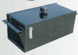
The 8.5 gallon box type reservoir is designed to be frame mounted. It hangs out of the way and is equipped with a brass wire mesh suction strainer, oil level & temperature gauge.
