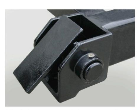
The hinges are cast from extra heavy duty 4140 grade steel to ensure durability. Adding to the ease of installation and durability, these hinges are welded directly to the body's main runners.
