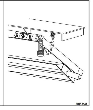
Waltco recommends that the C-Series liftgate be inspected at 6 month or 3000 cycle intervals to help assure proper function and operation of the liftgate.
