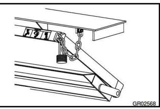
Inspect fold over assist spring and related hardware. Check that coiled pin (A) contacts and holds torsion spring when platform is unfolded open.
