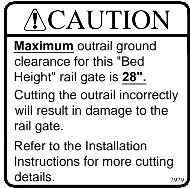
Decal No. 14 Located on the inside of each upright below the mainframe (BED HEIGHT GATES ONLY).
