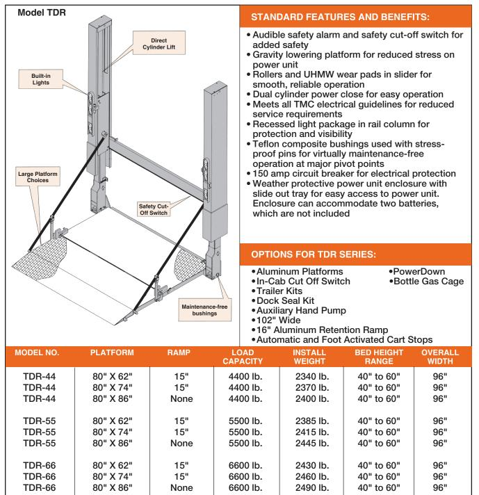
NOTE: Minimum bed height requirements for dock loading: 40" for 62" depth platforms, 45" for 74" and 86" depth platforms. All platforms listed above are two-piece folding. NOTE: Lower bed heights are possible depending on allowable ground clearance.
