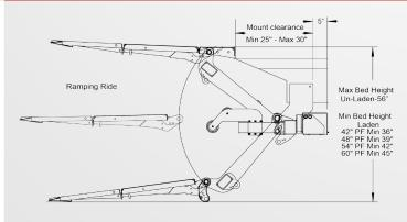
Designed to maximize your ROI, the PLR is perfect for city delivery applications and offers many new features like increased capacities up to 3,300 lbs., dual cylinders for added stability, large platform sizes in several configurations and walk ramp capabilities.
