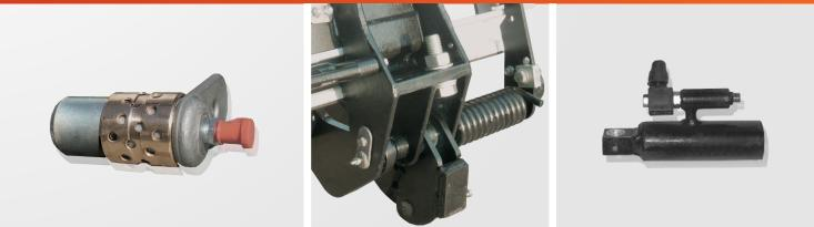
PALFINGER liftgates are built with oversized componets for greater reliability. Our liftgates feature heavy duty greasable pins and bushings, hydraulic cylinder locks and adjustable shim stacks for platform adjustment and torsion assist tuning.
