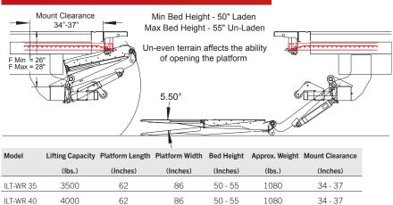
\*50" Min floor height is based upon a laden truck on flat ground with a 4" rear sill without insulation below the X-member
