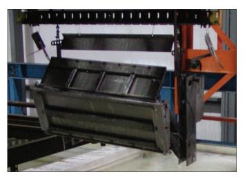
Every Pickup Lift is cleaned in a series of four baths then pre-treated with a phosphate conversion coating to prepare the lift for electro coating.
