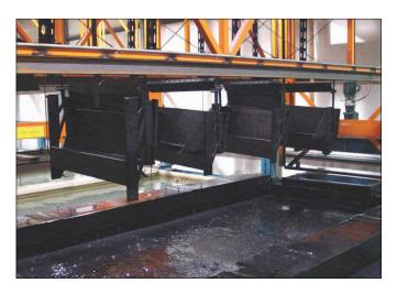
Once painted, the Pickup Lift is rinsed to recycle any undeposited paint, achieving nearly 100% paint efficiency for an environmentally friendly process.
