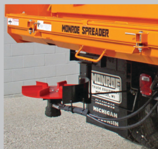
Standard Self Leveling Spinner with Stabilizer Rod
