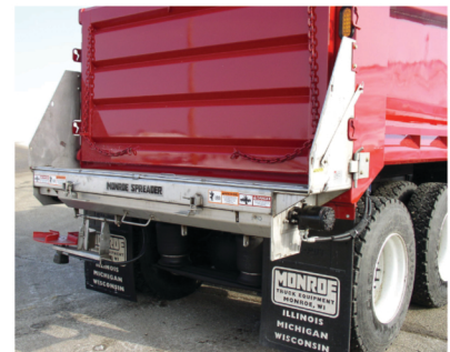
Optional Extended Side Shield Can Eliminate Internal Tailgate Spreader Shields
