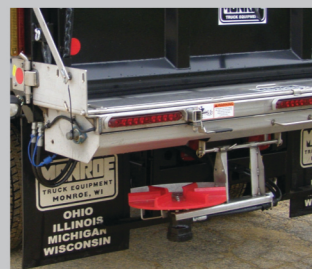
Self Leveling Spinner without Stabilizer Rod
