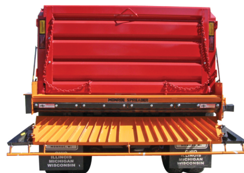
Optional Chip Attachment: Swing out chip spreader attachment for 11' chip coverage
