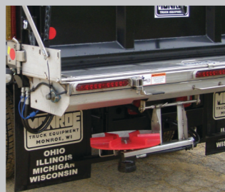
Self Leveling Spinner without Stabilizer Rod
