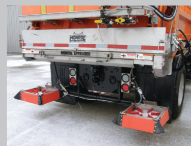
Stationary Bumper Mount Spinners on a One-Way Dual Discharge Spreader
