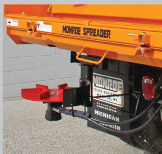
Standard Self Leveling Spinner with Stabilizer Rod
