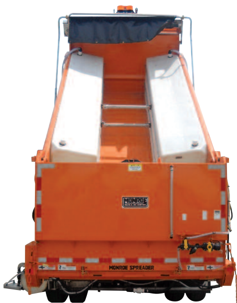
In-Bed Tank Pre-wet System
