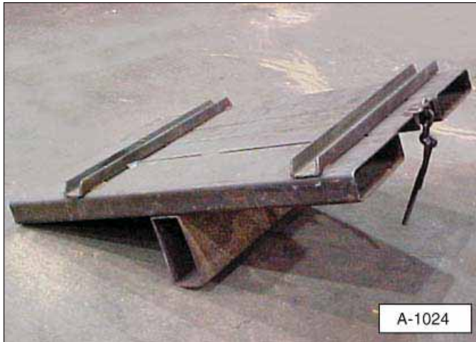
Installer-built Lifting Device.
