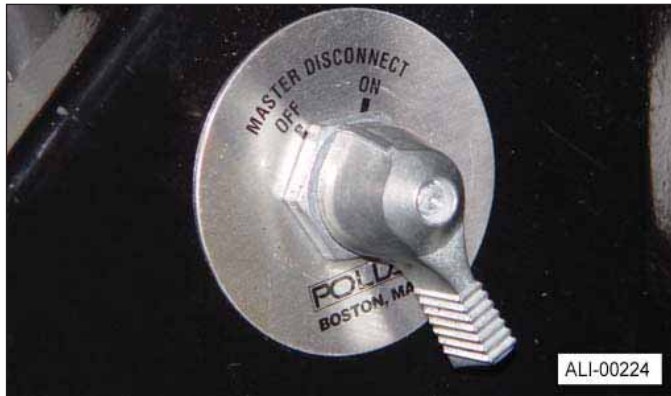
Cut-off switch mounted in cab of truck.
