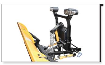
Streamlined appearance with an encased power unit that features adjustable drop speed and patented cable management system.
