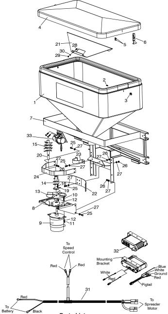
Note: Auger Extension (15) must be removed when using salt only. If it is not removed this may cause the motor to stall.
