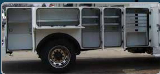
44.5" high compartments with large door clearance provide ample storage space and easy access to tools and equipment
