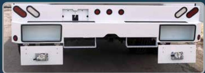
Optional storage bumper features dual lockable compartments, factory installed L.E. D. light kit, twin steps and recess for optional hitch package
