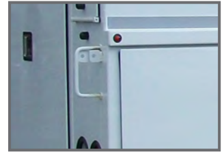
Masterlocking Steel Slide Bar – Simultaneously locks all of the side compartment doors. Spring loaded for easy manual operation.
