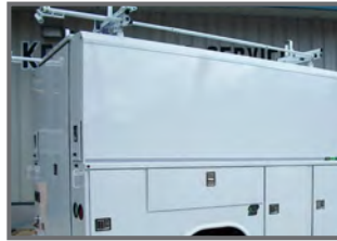
Roof-mounted single & dual pull-down assist ladder rack
