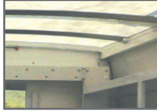
Optional Translucent Roof – Full translucent roof provides optimum visibility in all weather conditions.
