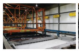
Components are cleaned and pretreated with a phosphate conversion coating to prepare the product for electrocoating.
