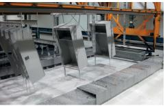
Components are removed from the bath and rinsed to reclaim any unset paint solids.
