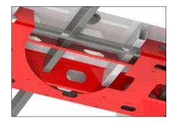
**HYBRID TORSION BOX**Eliminates truck frame and side pack deflection, 12ga grade 50 galvanealed
