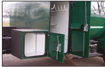
Standard reinforced door panels with durable 'T' locking latches
