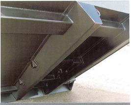
A bottom view of the 453U reveals the crossmemberless understructure with heated body option
